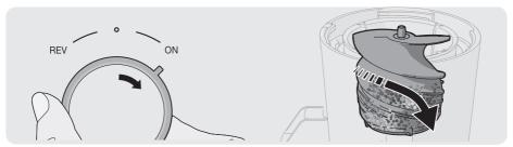
When the reverse motion comes to a complete stop, turn the power dial to the direction of [ON] (clockwise) to run.
